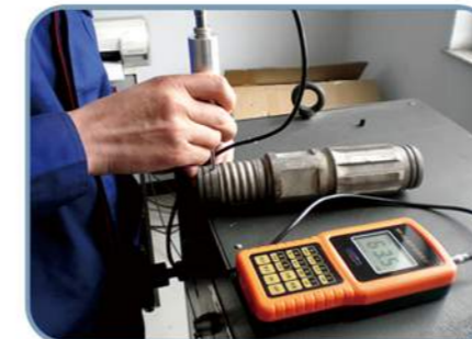
超声波硬度计检验 Inspection of ultrasonic hardness Test
