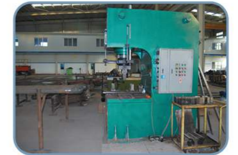
三点压力检验 Three Point Pressure Test
