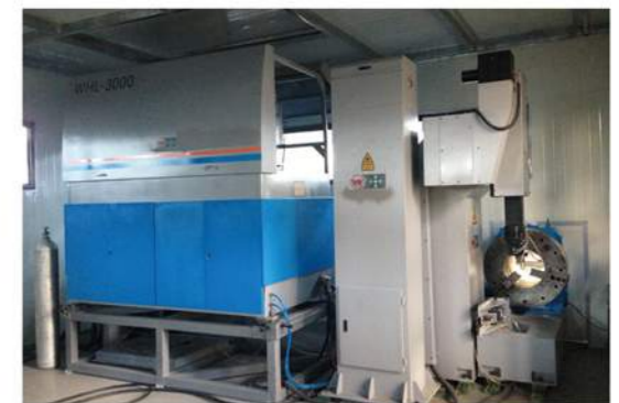
接头螺纹激光处理 Threaded joints laser treatment
